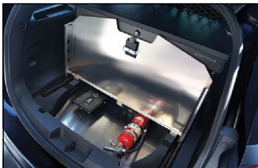
Setina's Easy-Lift Cargo Deck replaces the vehicle's factory rear compartment deck and provides a secure storage solution.
