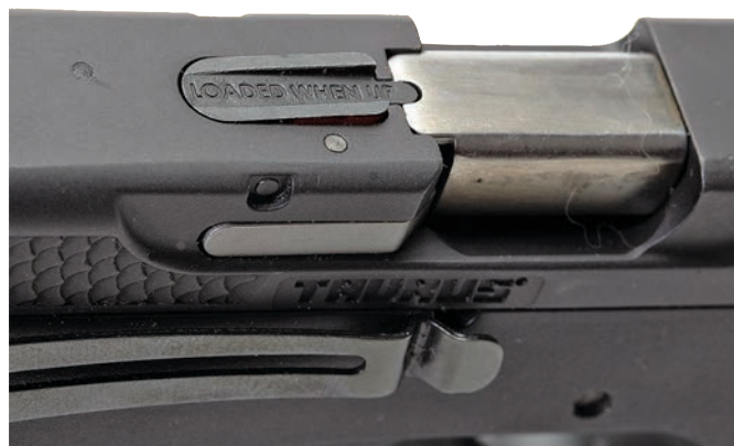
The Limited Chamber Indicator and sight is centered on the ample ejection port. The external spring powered extractor is lower right of the port. The belt clip is attached to the frame.
